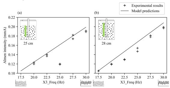
Fig. 9. Comparison between the linear model predictions from Equation (7) and validation Almen intensities data as a function of X3\_Freq. The other levels are shown in Table 2 and correspond to (a) MV01 to MV05 (X2\_Mass = 500 kg) and (b) MV06 to MV11 (X2\_Mass = 544 kg). The  $R^2$  value compares the experimental data and the DOE model predictions
