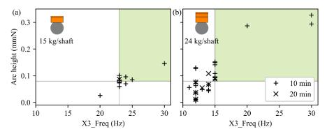
Fig. 4. The effect of X3\_Freq on arc heights of Almen N strips after vibratory peening for, (a) X1\_Ecc=15 kg/shaft and (b) X1\_Ecc=24 kg/shaft. For each test, X2\_Mass, X4\_Press, X5\_Depth and X7\_Lub were randomly varied. X6\_Pos was fixed at the centre
