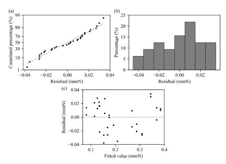
Fig. 7. Residues analysis of the screening model with primary effects on Almen intensity. (a) The aligned distribution of the residuals on the normal probability plot. (b) The histogram of the residuals centred at 0.(c) The residues as a function of the predicted values without specific pattern or general trend in the mean values
