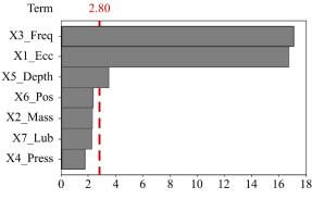
Fig. 6. Pareto chart of standardized effect of the primary factors on Almen intensity. Factors on the right of the reference line at 2.80 are statistically significant
