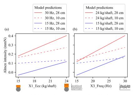
Fig. 10. Model profiler for the definitive empirical model. Almen intensities from Equation (7) are plotted as a function of (a) X1\_Ecc for the minimal and maximal values of X3\_Freq and X5\_Depth, (b) X3\_Freq for the minimal and maximal values of X1\_Ecc and X5\_Depth
