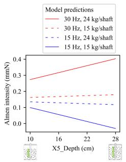
Fig. 11. Model profiler for the definitive empirical model. Almen intensities from Equation (7) are plotted as a function of (a) X5\_Depth for different tub energies, given by the levels of X1\_Ecc and X3\_Freq
