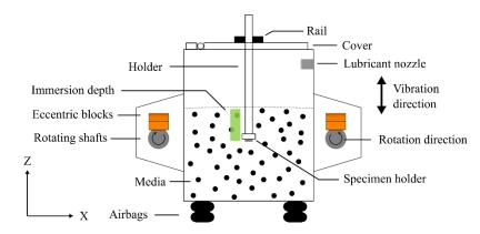
Fig. 1. Schematic representation of the vibratory peening machine showing a specimen clamped on the holder
