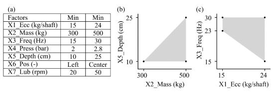
Fig. 3. Design of experiment method showing (a) the upper and lower levels of the seven process parameters and the restricted level variation range of (b) X5\_Depth as a function of X2\_Mass, and (c) X3\_Freq as a function of X1\_Ecc
